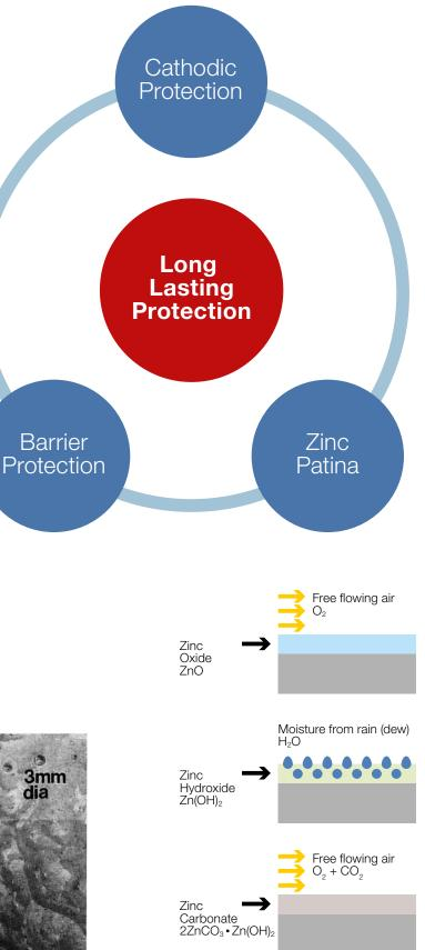
Above: The zinc patina begins its development with exposure to oxygen in the atmosphere. Moisture from rain or humid air reacts with this layer to form zinc hydroxide. This layer then reacts with carbon dioxide present in the atmosphere to form the tightly adherent, insoluble zinc patina.
