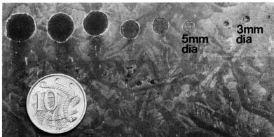
The galvanized steel test piece has had circular areas of the coating removed before exposure in a severe industrial environment. Sacrificial protection is provided by the surrounding galvanized coating and has prevented corrosion of the exposed circles up to 3mm diameter and minimised corrosion of the 5mm circle. Larger circles also exhibit corrosion-free annular areas adjacent to the surrounding coating.
