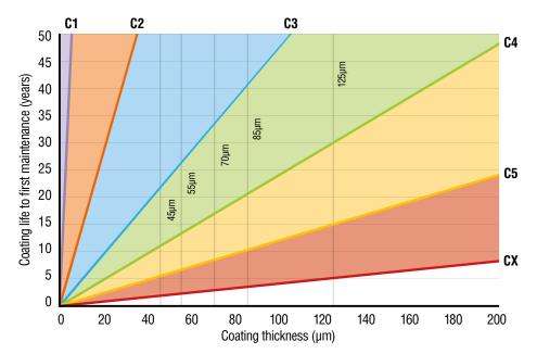
The chart shows that steel with an initial coating thickness of  $85\mu$ m in a C4 corrosivity zone will have an expected life to first maintenance of 20 - 40 years.
