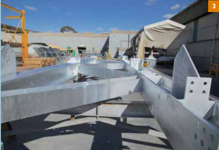
(3) the completed article showing slight marking at the intersection of the dips, which will fade in time.
