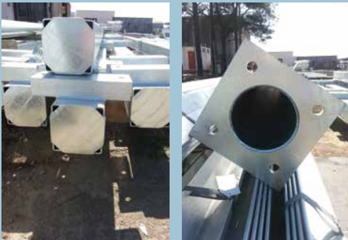
Vent holes can be drilled or cropped to allow the zinc to drain from the inside of hollow sections. The best venting for hollow sections for quality will allow the zinc to freely flow through the article.
