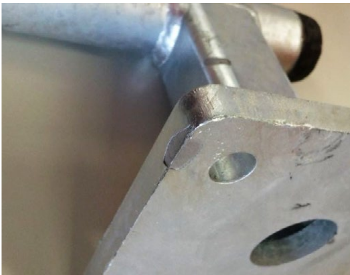
FIGURE 5: Flaking of coating at a laser cut edge
