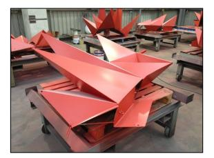
The paint work component involved whip blasting surface preparation, before applying a prime coat of DUREMAX<sup>®</sup> GPE at 75 microns and a topcoat of WEATHERMAX<sup>®</sup> HBR of 50 microns thickness.
