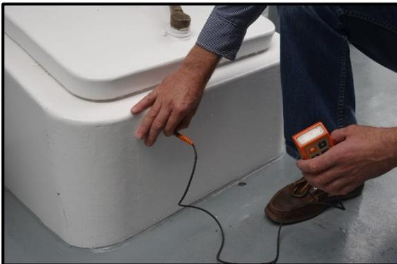
A hatch body with 743  $\mu\text{m}$  of duplex coating
