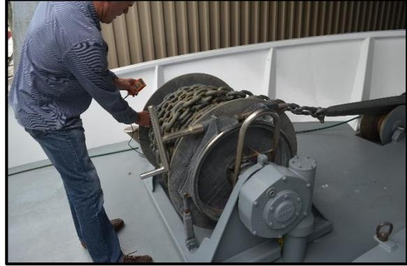
Anchor spool with 220  $\mu\text{m}$  of HDG coating
