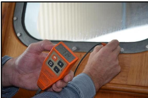
Inside the wheelhouse and a window frame HDG coating of 114 $\mu$ m
