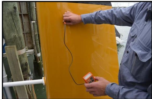
A funnel cover with 848  $\mu\text{m}$  duplex coating
