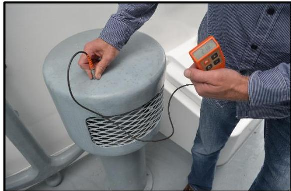
Vent with 218  $\mu\text{m}$  of duplex coating
