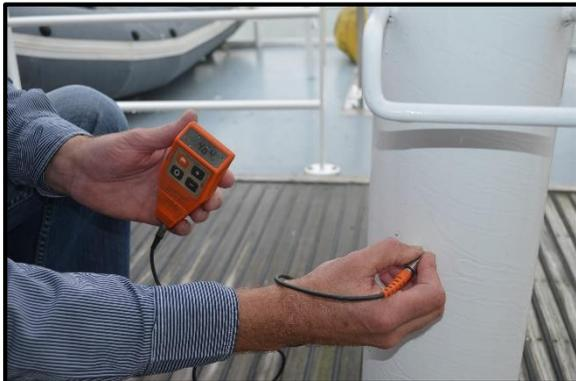
The mast with 464 $\mu$ m of duplex coating
