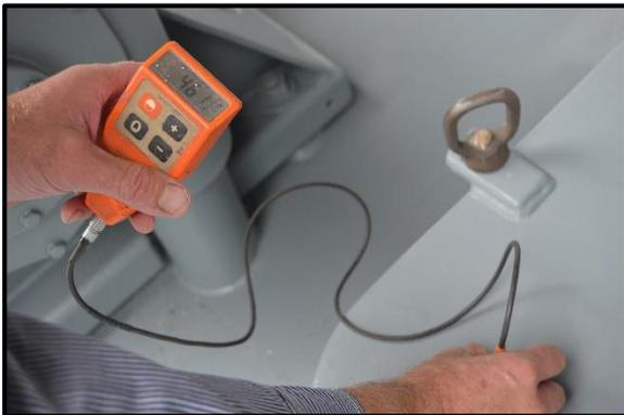
A hatch cover with 461  $\mu\text{m}$  of duplex coating
